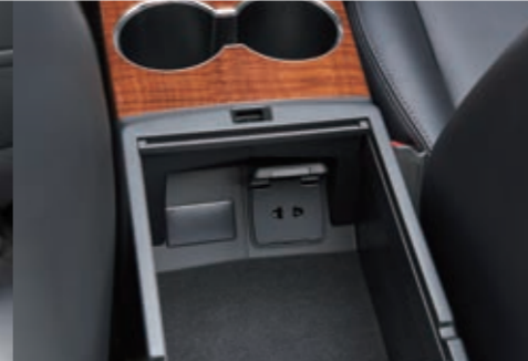
AC power outlet Simply plug in to power small electric devices up to 150W. Note: The maximum voltage and plug type may vary depending on market model.
