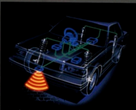
Nissan's ultra-sophisticated electronically controlled suspension automatically alters its damping rate in accordance to road and running conditions.
