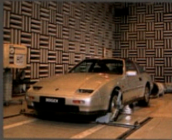
Anechoic room test
