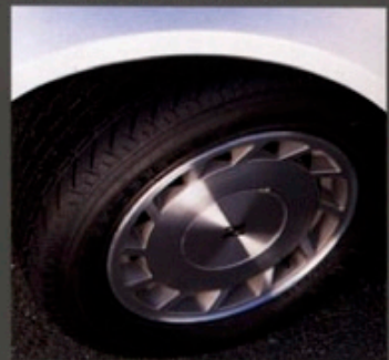
215/60VR15 radial tires on 6-1/2JJ x 15 alloy wheels
