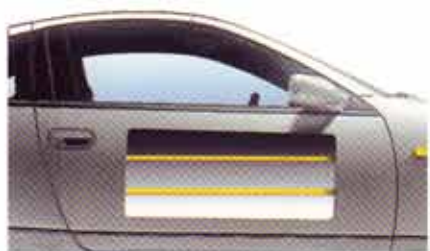
The introduction of side door guard bars dramatically reduces the effects of side impacts.
