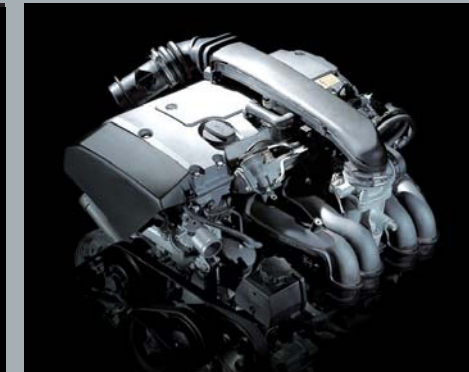
149.5ps(110kW) 2,295cc 2.3L petrol engine
