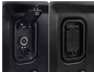
Deck power outlet
