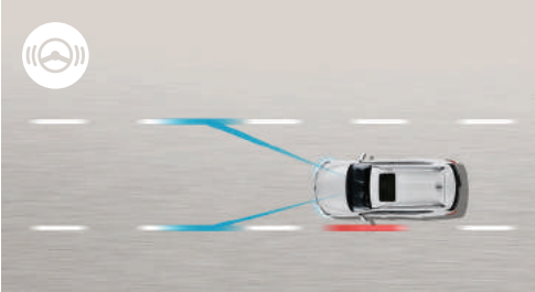
Lane Keeping Assist (LKA) With the front view camera, the system automatically operates the steering wheel to prevent departure whenever the vehicle begins to depart from the lane without turn signal activation. Operating condition : above 40 km/h
