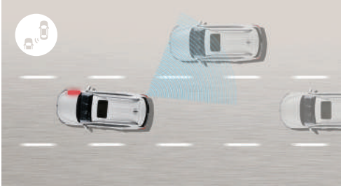
Blind Spot-Collision Assist (BSA) If the collision risk in the rear blind-spot increases when a driver approaches the lane for a lane change, it helps to avoid collisions by differential braking.
