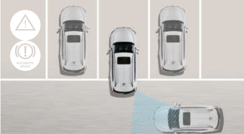
Rear Cross Traffic-collision Assist (RCTA) When backing out from a parking space, the RCTA detects approaching vehicles from the left or right direction. After detection, the system gives alert and initiates braking maneuver if necessary.
