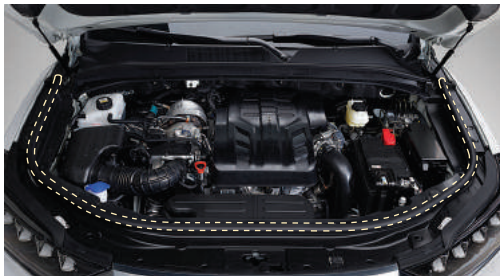
Engine room around sealing cover
