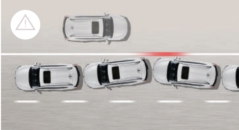
Driver Attention Warning (DAW) If the DAW system senses the driver's attention level has been significantly reduced, it will give audible warning and graphic on cluster.
