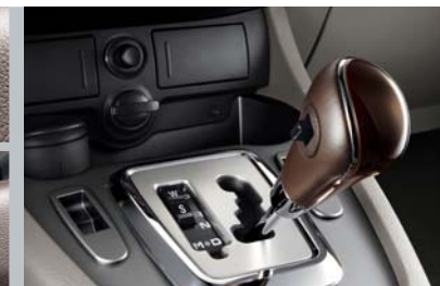
5-speed E-Tronic automatic A built-in AI programme to predict the driver's driving habits and assess vehicular status for optimal gear-shifting performance. The Tip Switch provides the responsiveness of a manual transmission, while the Winter Mode enables starts in 2nd gear, preventing slippage on ice or snow.
