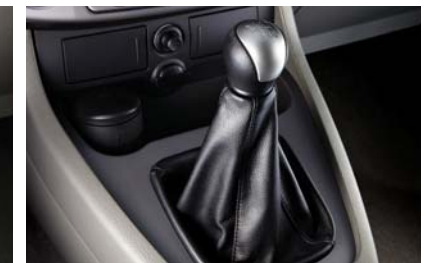
6-speed manual The wide gear ratio provides more power when starting out and lowers the engine rpm at high speed, for less noise and better fuel efficiency. Self-adjusting technology and concentric slave cylinder extend durability and help to maintain firm pedal force.
