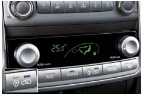
Air quality control system (keeps noxious fumes out)
