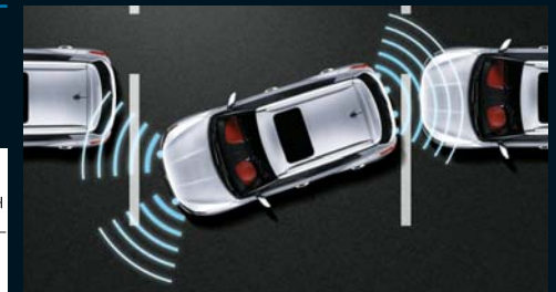
Outside parking sensors and camera in rear
