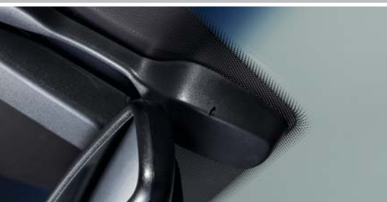
Rain sensing and automatic light control unit
