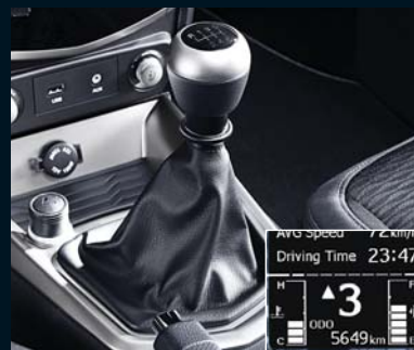
6-speed manual transmission (with gear-shift indicator)
