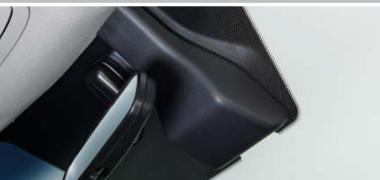
Front camera module (AEB/LDW/LKS/HBA/TSR) with rain sensing and automatic light control unit
