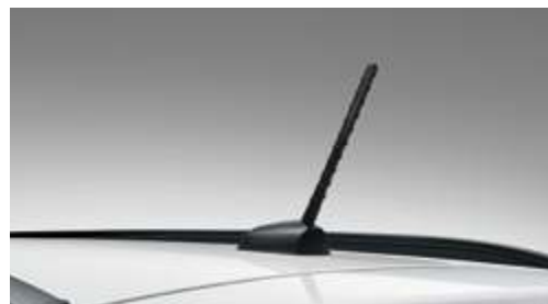
Roof-mounted pole antenna
