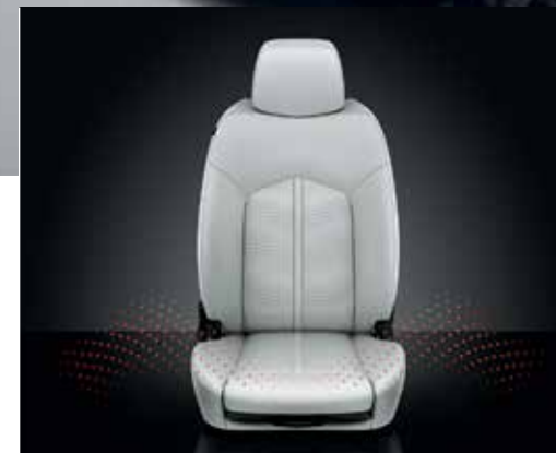
SAFETY ALERT SEAT The available patented Safety Alert Seat intuitively sends subtle pulses through the seat cushion, left or right or simultaneously, alerting you to a variety of potential hazards on the road.
