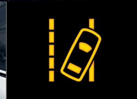
LANE DEPARTURE WARNING Offering the latest innovation in driver awareness, available Lane Departure Warning issues visual and audible warnings as well as subtle pulses through the seat cushion if the vehicle begins to drift out of its lane without the driver first activating the turn signal.
