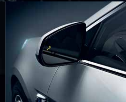
SIDE BLIND ZONE ALERT Available Side Blind Zone Alert 3 uses radar-equipped sensors that sweep the sides of the SRX. If your turn signal is activated and a vehicle enters one of your blind spots, an alert warns you of its presence. It's like having an extra set of eyes so you can more safely change lanes.
