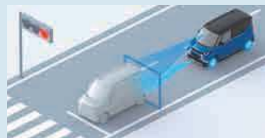
FCM = Forward Collision Mitigation system
