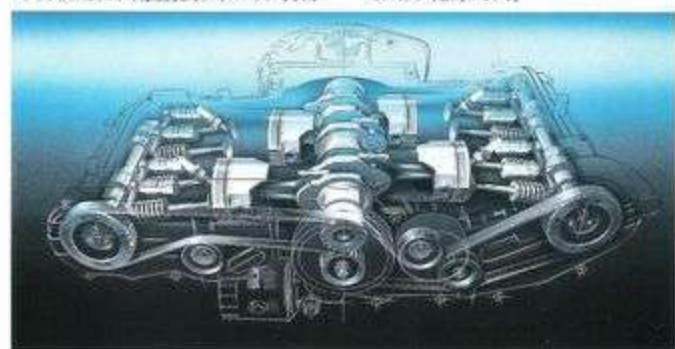
FLAT-4 Turbocharged FLAT-4 Engine with EGI System
