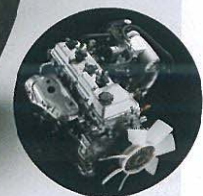
LASRE α-II 3RZ-FE 16VALVE EFI Displacement : 2,693ℓ Maximum Power (NET) : 110kW (150PS) / 4,800 r.p.m. Maximum Torque (NET) : 235N·m (24.0kg·m) / 4,000 r.p.m.
