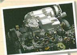
LASRE 3C-TE DIESEL TURBO piston displacement: 2,118cc maximum power: NET 66kW (94 PS)/4,000 r.p.m. maximum torque: NET 209N-m (23.0 kg-m)/2,000 r.p.m.
