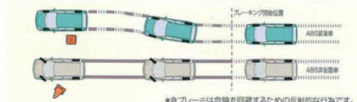
ABS:Antilock Brake System
