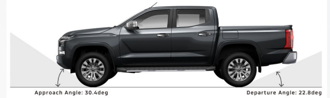
Approach Angle and Departure Angle
