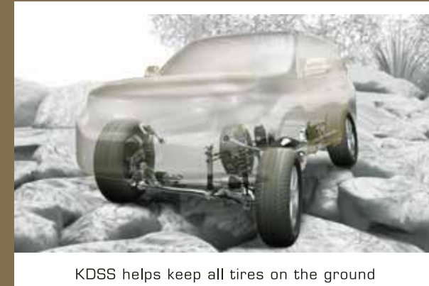
KDSS helps keep all tires on the ground
