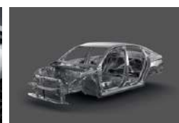
BODY Sturdy GOA body Effectively absorbs impact of collision
