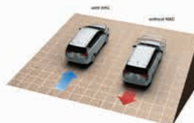
Hill Start Assist Control The HAC system helps increase control on steep slopes and prevent individual wheels from locking
