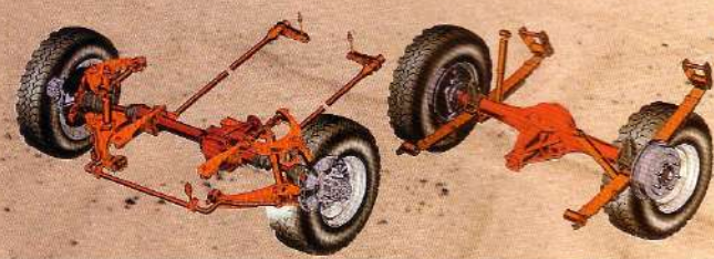
Independent double wishbone front suspension / ventilated disc brakes (left) Semi-elliptic leaf spring with bias-mounted telescopic shock absorbers rear (right)
