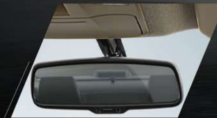
Automatic electrochromic rear view mirror.
