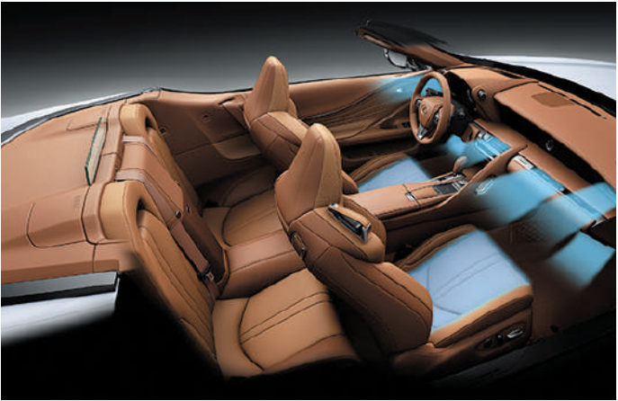
Lexus Climate Concierge The Lexus Climate Concierge automatically controls the cabin temperature, seat heaters and Ventilated Seats for the front seats. It realises different control settings depending on whether the soft top is open or closed. When the soft top is open, in addition to the control settings for when the top is closed, the Concierge responds to the vehicle's speed, optimising the temperature to embrace occupants in a refined and relaxing environment.
