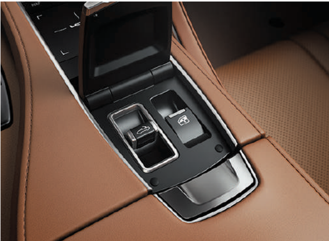
Roof Switch In a subtle Lexus refinement, the soft top control switch is concealed under the palm rest, creating a special feeling of opening the lid that mimics opening/closing the soft top. For intuitive operation, the switch direction matches the movement of the roof. The switch features a non-slip Lexus L-shaped pattern, providing tactile feedback for confident operation.
