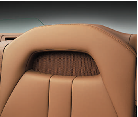
Mark Levinson Audio System The audiophile-quality Mark Levinson Reference Surround Sound System incorporates an 11-channel amplifier that drives 13 speakers, including speakers integrated into the rear seat headrests, to replicate a precise sound stage that reproduces the position and depth of each instrument. When the soft top is open, the system automatically complements and adjusts the sound architecture in real-time to deliver the audio quality you enjoy with the soft top closed in an open-air environment, and harmonise with the sound of the engine.
