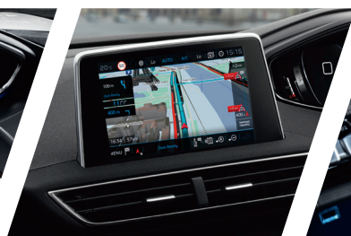
Latest generation 8" capacitive multifunction colour touchscreen
