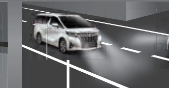
Automatic High Beam (AHB)* Automatically switches between high beam and low beam as needed to provide maximum road visibility.
