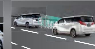
Dynamic Radar Cruise Control (DRCC) for All Speeds* Maintain a safe distance with preceding vehicle and brakes automatically when the car ahead stops.
