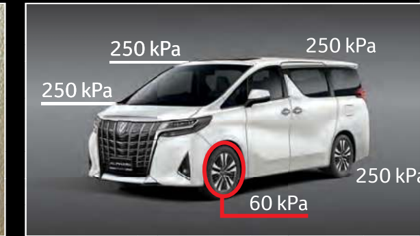
TYRE PRESSURE MONITORING SYSTEM (TPMS) Displays real-time tyre pressure information via multi-information display (MID). Alerts driver when tyre pressure is below ideal level.
