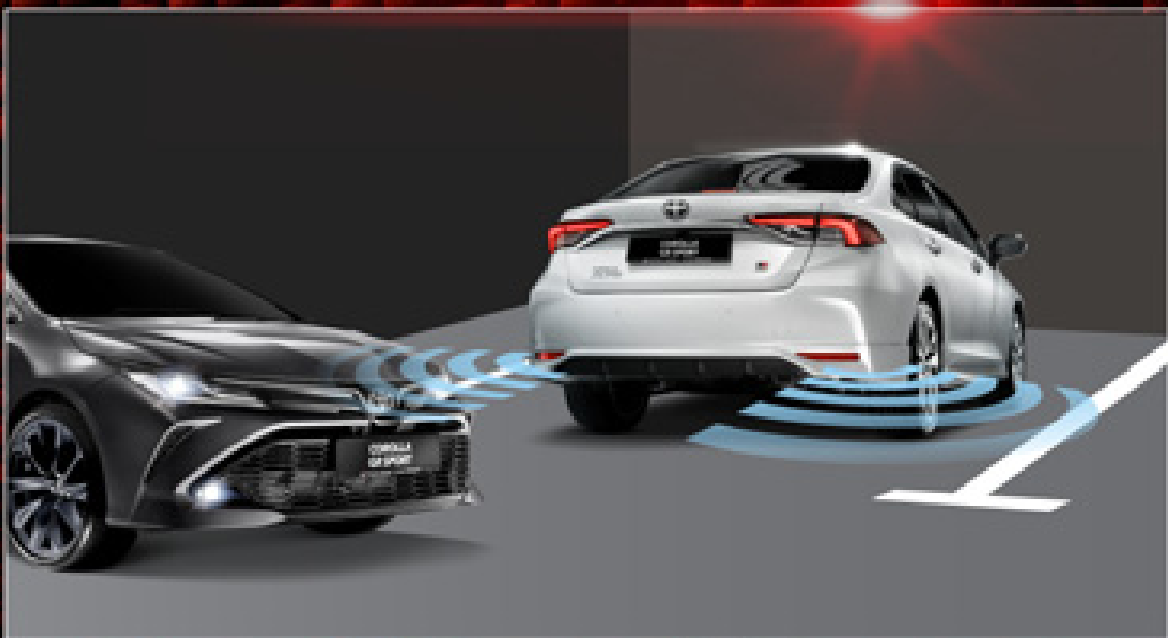
Rear Cross Traffic Alert (RCTA)* Using radar sensors to detect approaching traffic, the system alerts the driver through audio alerts and flashing side mirror indicators if a vehicle is detected.
