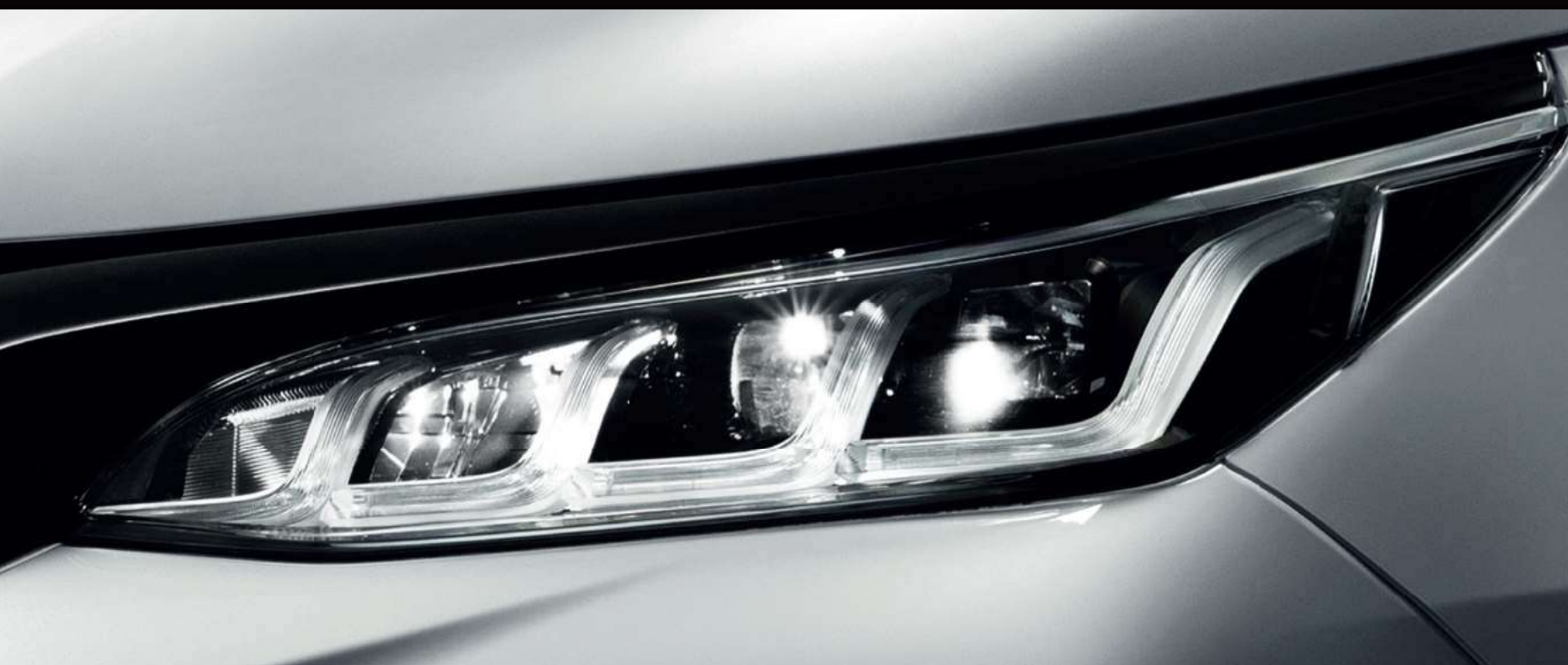
New Quad LED Headlamps with LED Daytime Running Lights Greater sight and visibility for both night and day.
