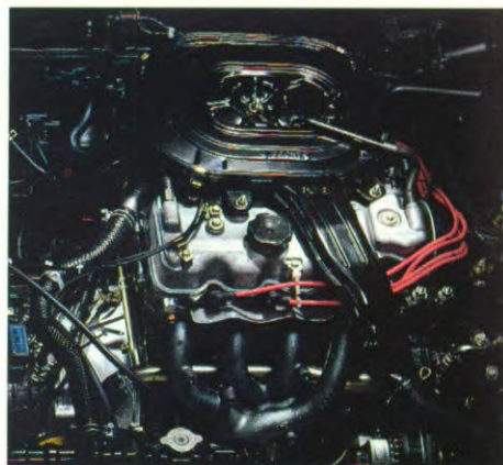
2.0 liter benzinemotor (vermogen 75 kW/6000 rpm)
