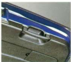
An excellent example of the uniform utility that is absent from many other station wagons is the interior tailgate handle, which enables closing the tailgate without touching the tailgate's exterior surface.
