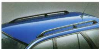
The convenient roof rails are an elegant styling touch, while greatly simplifying the attachment of ski racks, roof racks and other accessories.
