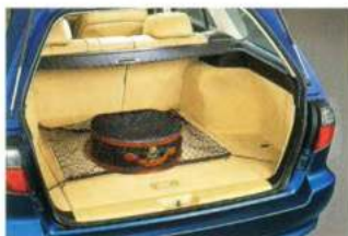
An extra-strong net plus conveniently located floor- and wall-type hooks, let you securely anchor bulky luggage and other gear.
