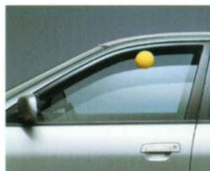
Anti-trapping power window
