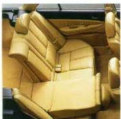
Folding down either side of the Station Wagon's 6:4 split rear seat permits the carrying of long, bulky or oddly shaped items.
