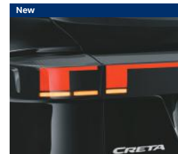
LED rear turn signal with sequential function
