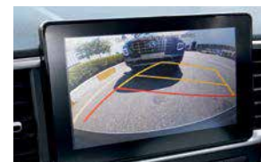
Rear Parking Assist System
