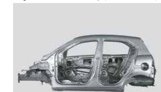
High Structural Safety (AHSS & HSS)
