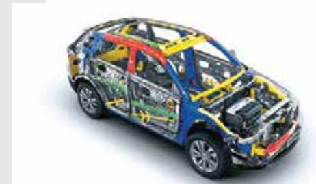
Reinforced Safety Structure Utilising hot press forming (HPF) method of metal stamping that results in increased strength and rigidity compared to normal metal stamping.
