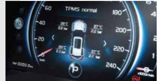
Tyre Pressure Monitoring System (TPMS) Monitor real time tyre pressure and temperature to provide peace of mind.
