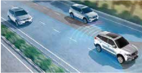
Blind Spot Information System (BLIS) * Monitor for blind spots and alerts the driver when vehicles are nearby.
