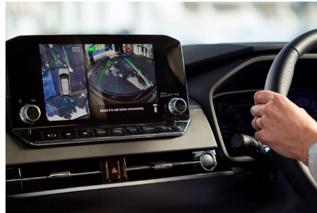
» SAFETY FROM EVERY ANGLE The Multi-Around View Monitor gives you an all-round view for safety in tight spaces (VRX only).
