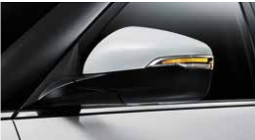
LED repeaters on exterior mirrors
