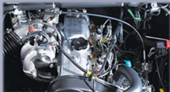
Powerful yet Economical 4D56 which is now Euro-2 Compliant 2.5L 4 In-line Diesel Engine, Distributor Type Fuel Injection
