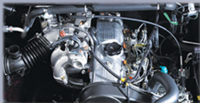
Powerful yet Economical 4D56 which is now Euro-2 Compliant 2.5L 4 In-line Diesel Engine, Distributor Type Fuel Injection
