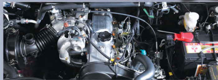
Powerful yet Economical 4D56 which is now Euro-2 Compliant 2.5-Liter 4 in-Line Diesel Engine, Distributor Type Fuel Injection
