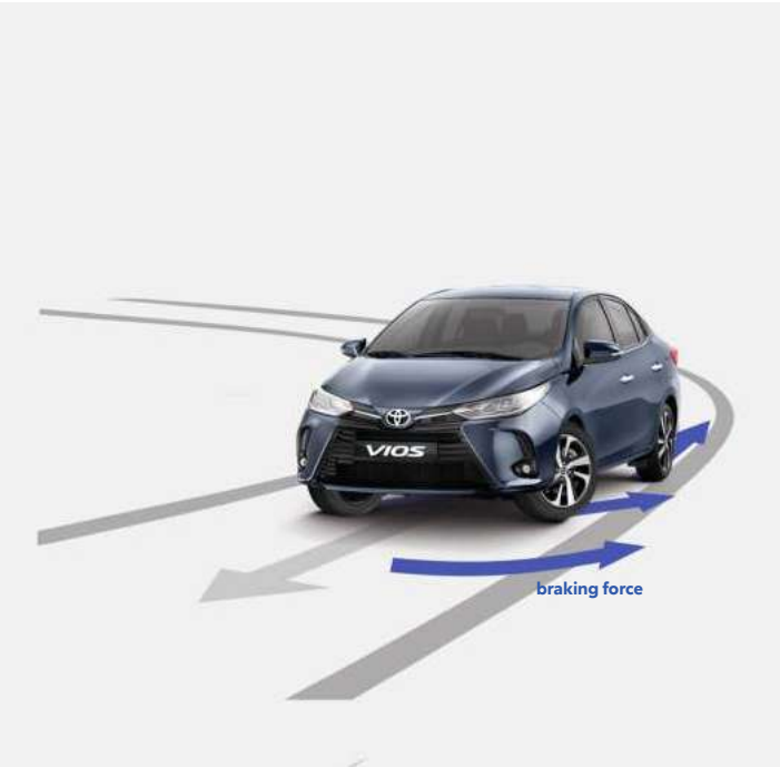
ELECTRONIC BRAKE DISTRIBUTION WITH BRAKE ASSIST This feature intelligently transfers most of the braking to the wheels that have more grip and provides additional brake force when the car needs to make an emergency stop.
