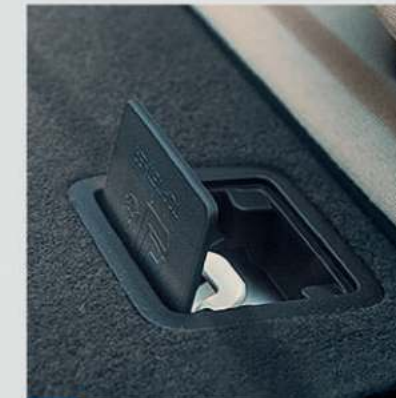
ISOFIX Anchor Points Are situated behind the rear seat head rest.
