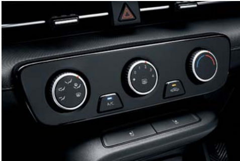
Manual air conditioning system
