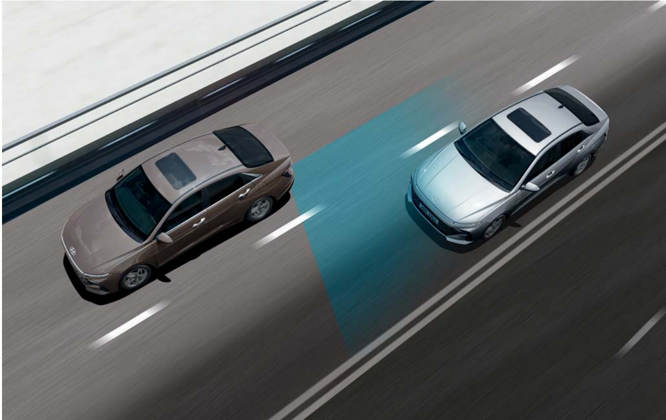
Blind Spot Collision Avoidance Assist (BCA) BCA uses radar to monitor both of your blind spots. If a vehicle is detected in the blind spot while the turn signal is flashing, BCA will automatically apply left or right side front braking before your attempted lane change thus helping you avert an unsafe lane change and a potential collision.
