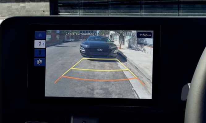
Rear Occupant Alert (ROA) When exiting the vehicle, instrument cluster icon flashes and warning chimes to remind driver of rear seat status. Rear View Monitor (RVM) For safer parking, a high-definition camera monitors the situation behind, and includes a graphic overlay to assist with parking.
