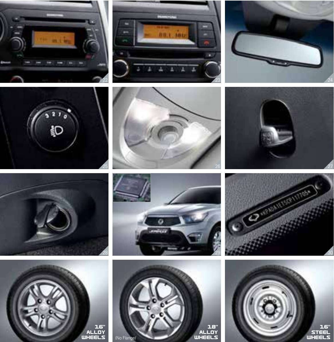
22/ 2-DIN AUDIO SYSTEM WITH MP3 AND CD PLAYERS 23/ RDS AUDIO SYSTEM 24/ ELECTROCHROMATIC REARVIEW MIRROR Darkens when hit by the headlights of tailing cars at night, preventing glare and enhancing driving safety. 25/ HEADLAMP LEVELLING DEVICE Adjusts the headlamps to prevent drivers in front from being dazzled by the light. 26/ CABIN LAMPS One-touch switches for ease of operation, designed to add elegance to the interior. 27/ SHOPPING BAG HOOK Helps to manage shopping bags inside. 28/ POWER OUTLETS Under the front passenger's seat and in the cargo bay. 29/ BATTERY SAVER Automatically turns off head lamps left on after the driver exits the vehicle. 30/ VISUAL VEHICLE IDENTIFICATION NUMBER PLATE (EU REGION ONLY)
