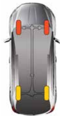
SNOWY & ICY INCLINES 50:50 torque distribution front and rear (4WD Lock)
