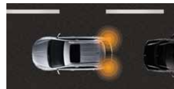
EMERGENCY STOP SIGNAL (ESS) It warns vehicles at the rear of emergency stops and ABS activation.
