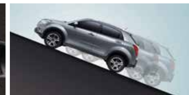
HILL START ASSIST (HSA) It's sometimes tough pulling away when you're facing uphill. HSA minimizes backward rolling on steep ascents.
