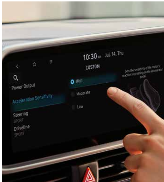
EV Performance tune-up Driver can adjust motor power, acceleration sensitivity, steering effort and driveline mode to meet their driving style.
