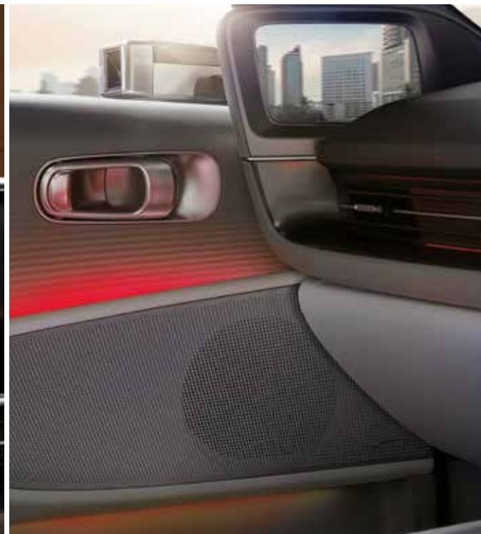
Speed Sync Lighting Brightness of front cabin lighting shifts from 10% at 30km/h to 100% at 100km/h, providing a dynamic driving experience.
