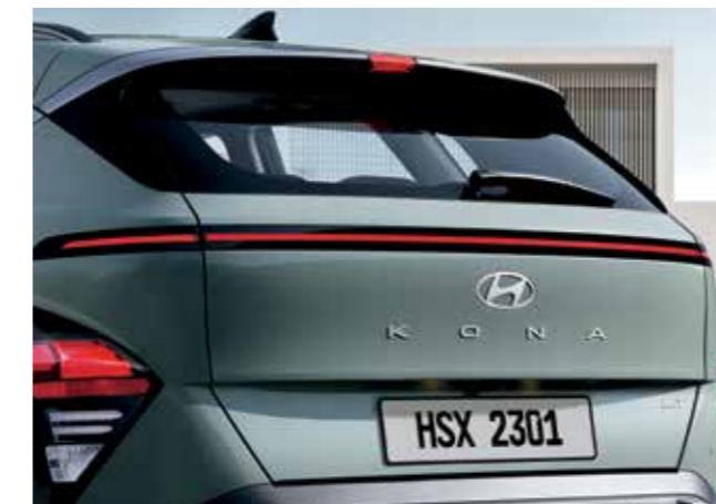
Spoiler Integrated HMSL, rear seamless horizon lamp, LED brake lamps, LED turn signal lamps
