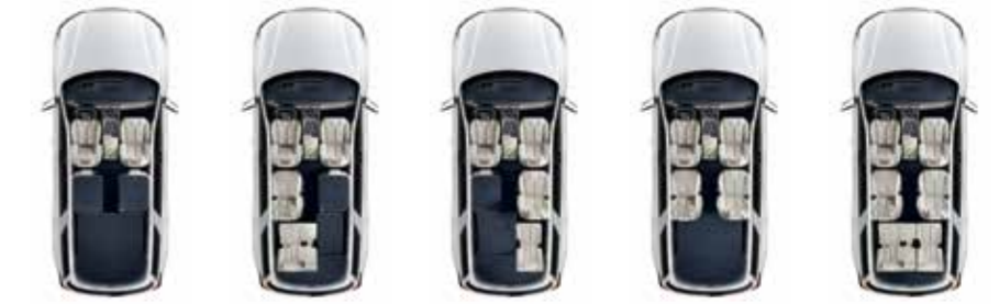
2nd and 3rd row folded 3rd row folded and 2nd row folded 60% 3rd row folded and 2nd row folded 40% 3rd row folded 7 seats
