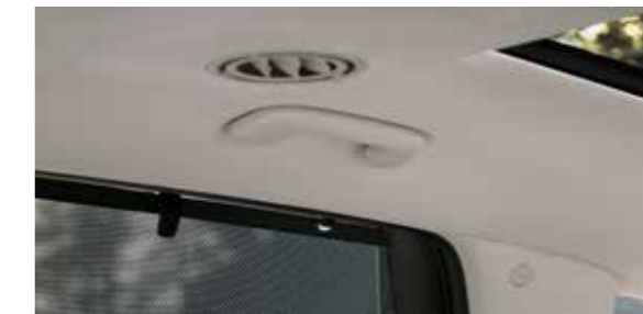
Standard rear air vents Innovative rear air vents keep air flowing and allow rear passengers to select between a focused, partially diffused and fully diffused stream of air.
