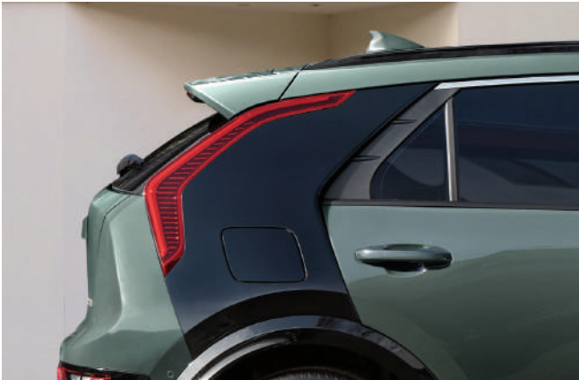
C-pillar air intake The C-pillar design highlights the profile of the car. To prevent static pressure, the aeropillar has an opening to let airflow through.
