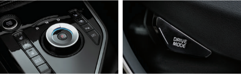
Shift By Wire (SBW) (SX only) Dial-type SBW provides superb operational convenience and safety in terms of console and indoor space utilization, as well as automatic P-Mode engaging logic.
