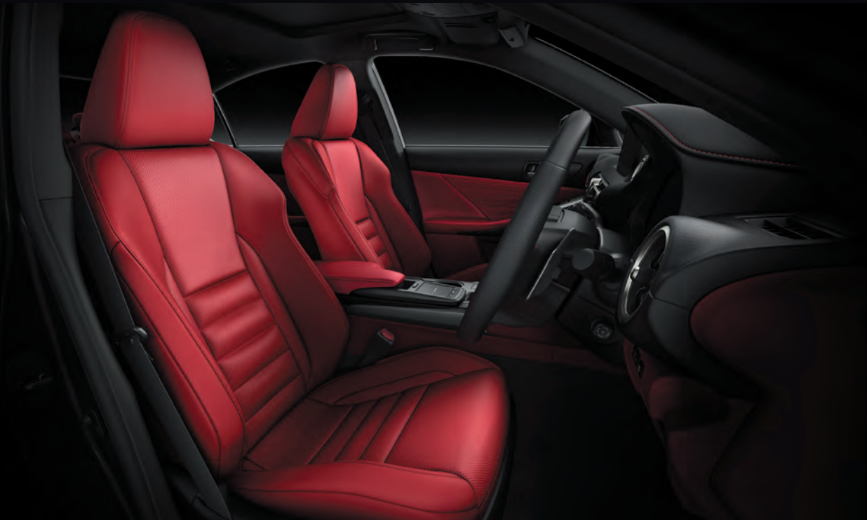
F SPORT front seats The front sports seats are the product of an innovative ‘integrated foaming’ manufacturing process. They provide a blend of refined comfort with firm support and excellent holding performance for sports driving.
