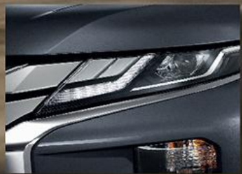
BI-LED PROJECTOR HEADLAMPS WITH LED DAYTIME RUNNING LIGHTS
