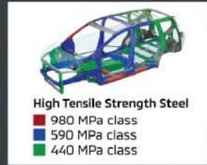
High Tensile Strength Steel 980 MPa class 590 MPa class 440 MPa class
